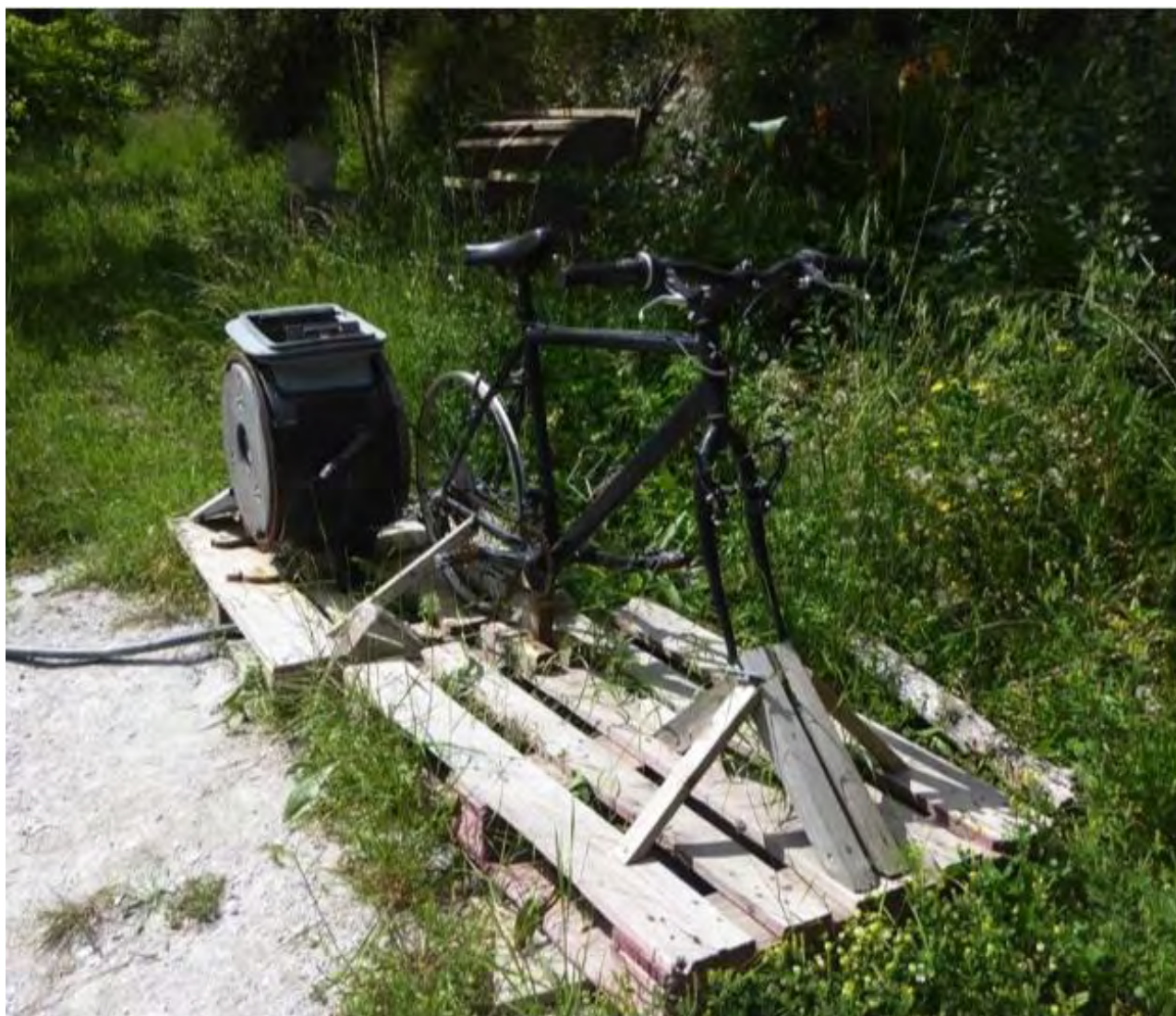
Non-electric washing machine, La Burra Verde, OST2018. Photo by Tim Whitworth
