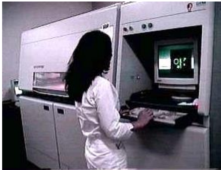
A Selective Laser Sintering machine being used at the Centro Renato Archer in Brazil. Image by R Sabbatini at English Wikipedia
