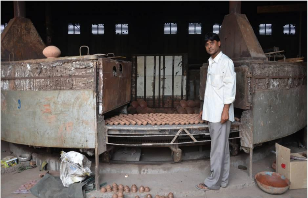
Mansukhbhai Prajapati with his semi-circular kiln for hardening clay products in Vakaner, Gujarat (Image: SRISTI)
